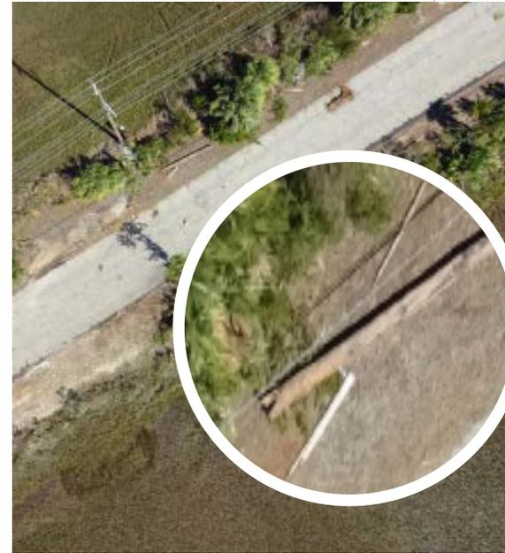
*Damage to telephone poles clearly visible from the air. Photos like these were used to identify areas where infrastructure was damaged. Once identified, a location like this one would be tagged with exact coordinates, helping Comcast technicians to quickly locate the downed lines.*
