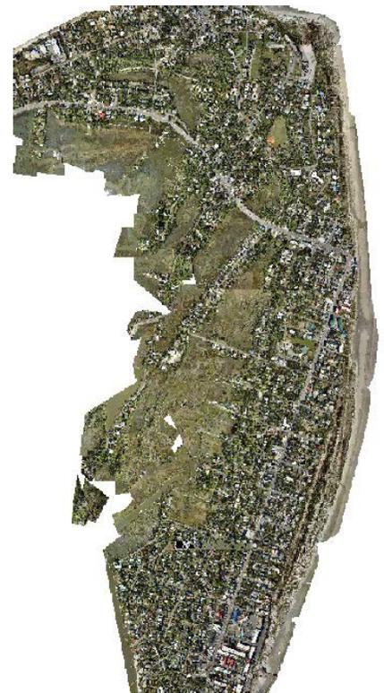
*The full orthomosaic created from a series of flights over Savannah, GA. For speed, each tile is analyzed individually for damage before being combined into a larger image.*
